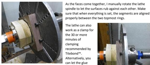
settle for 10 minutes and then move the bowl to another clamping system to free up your lathe while the glue hardens. Or, if you are in a hurry, you can mount another ring.
