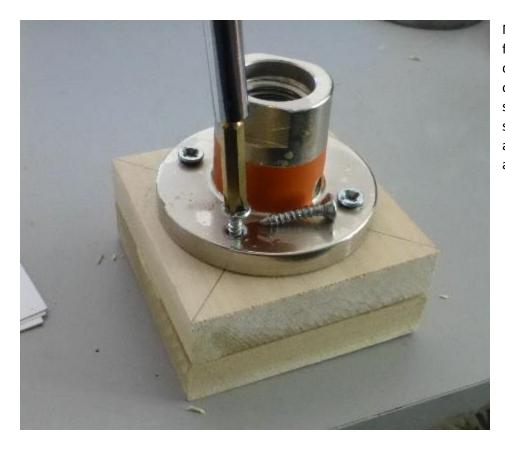
Mount the block to the flange after the glue is dry. For this I use 1" oval head sheet metal screws. Do NOT use sheetrock screws. They are notoriously brittle and break easily.
