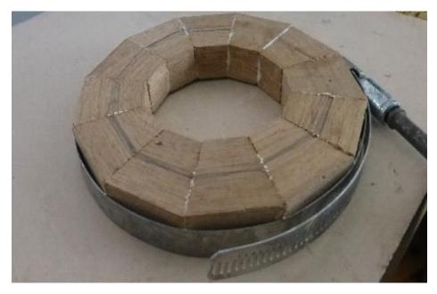
When all the segments have been glued, use a hose clamp to secure the ring. Tighten the clamp. This will often correct what initially appear to be errors. I use a 5/16" drive in a variable speed drill to tighten the clamp.
