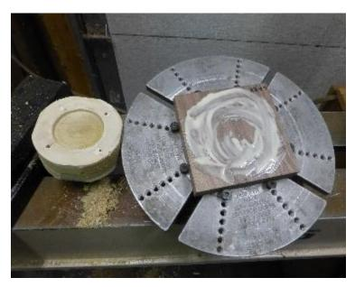
Put glue onto the faces to be glued.
