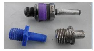
The photo shows a Live Tailstock Adapter (available from PSI Woodworking) on the top. The bottom images are fixed tail stock adapters. I made the smaller one (1" x 8tpi) with a 3D printer. The larger one (1 ¼" s 8tpi) is available from Amazon.
