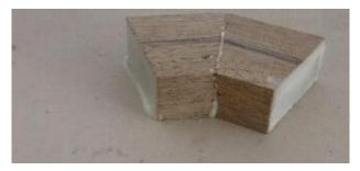
Then apply glue to the ends of a third segment and glue that to the left side. (11 o'clock position).
