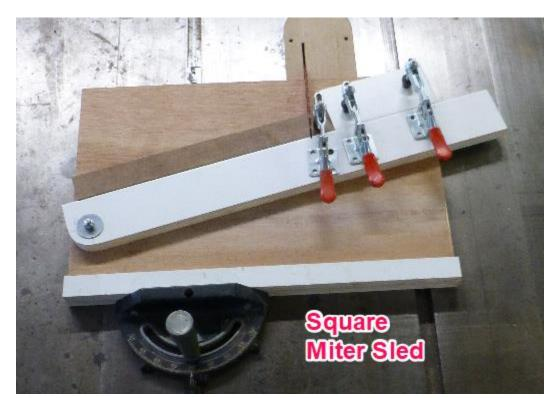
To make this sled, start with the following pieces cut from high quality  $\frac{3}{4}$ " plywood:
