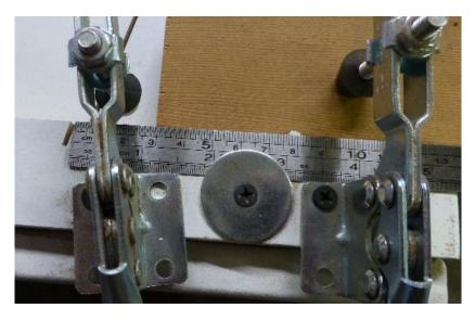
To calibrate the ruler, I start by putting the stop block to cut a segment of about an inch or so. I cut the segment. I then measure the segment in cm. I then set the ruler to the measurement that I got on the segment. This is rather "backwards", but it is much easier.
