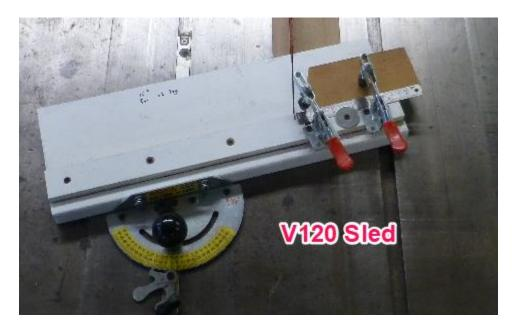
Start with a piece of high quality  $\frac{3}{4}$  inch hardwood plywood 6" x 18". Cut another  $\frac{3}{4}$  inch piece that is 2" x 18". Screw, clamp and glue the 2" board to the 6" board.
