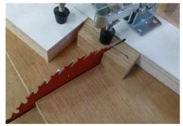
The accompanying photo shows the cutting of the last segment from stock that is just long enough. Notice that the segment is clamped in place. No fingers are anywhere nearby. It took just a second or two to set up this cut which I did with the segment well away from the blade.
