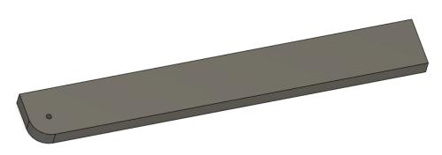
Secure the guide bar to the base using a  $\frac{1}{2}$ " bolt. Secure it with a nut – preferably a wing nut. Tighten it enough so that you can move the reference bar but it will stay where you set it.
