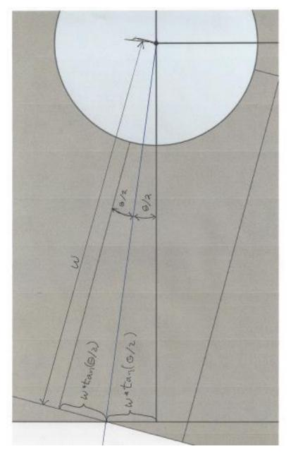
When you adjust the angle legs, this has the effect of shortening the lower leg and extending the upper leg. The amount of lengthening or shortening is the amount of offset of the hole from the edge of the meterstick times the Tangent of half the angle. This is shown to the left. (Sounds simple, right?)
