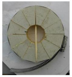
have closed. If not, redo this with larger or smaller shims as required or adjust the shims in the gaps to make it happen. Once you are satisfied, tighten the clamp and let the glue harden for 6 or more hours.
