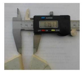
Alternatively, I could have turned the segment backwards and measured the difference between the segment and the space which in this case shows .191" of error.
