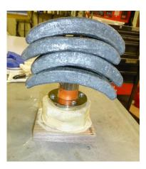
A large Bench Vice works well for small bowls. Be sure to include a board under the ring to assure even pressure over the entire ring.
